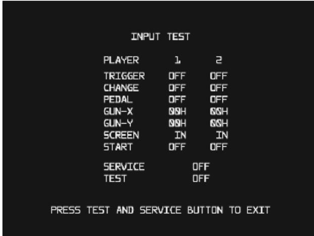
Selecting the INPUT TEST on the game test mode menu screen causes the screen (on which each switch is tested) to be displayed. Press each switch. If the display beside each switch indicates "ON," the switch and wiring connections are satisfactory.
