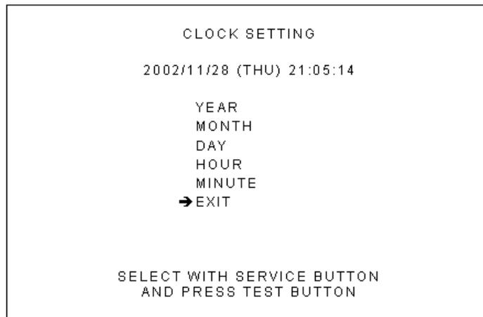
(1) Move the cursor to the desired item and press the TEST Button to increase values.
