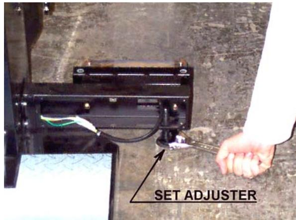
5. Attach the pedal to the foot base using 4 hexagonal bolts. Be sure not to tighten the hexagonal bolts completely.
